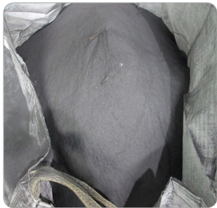
Metal Oxide Dust generated by Acid Regeneration
